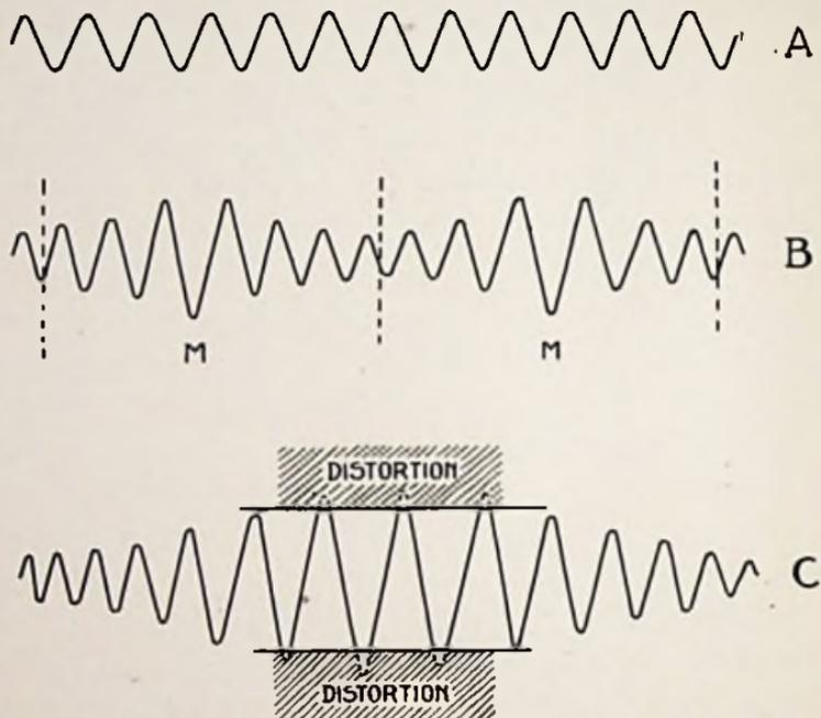
Fig. 5.—Cause of Distortion. A, Steady-carrier Wave. B, The Modulated-carrier Wave. C, Distorted Reproduction
