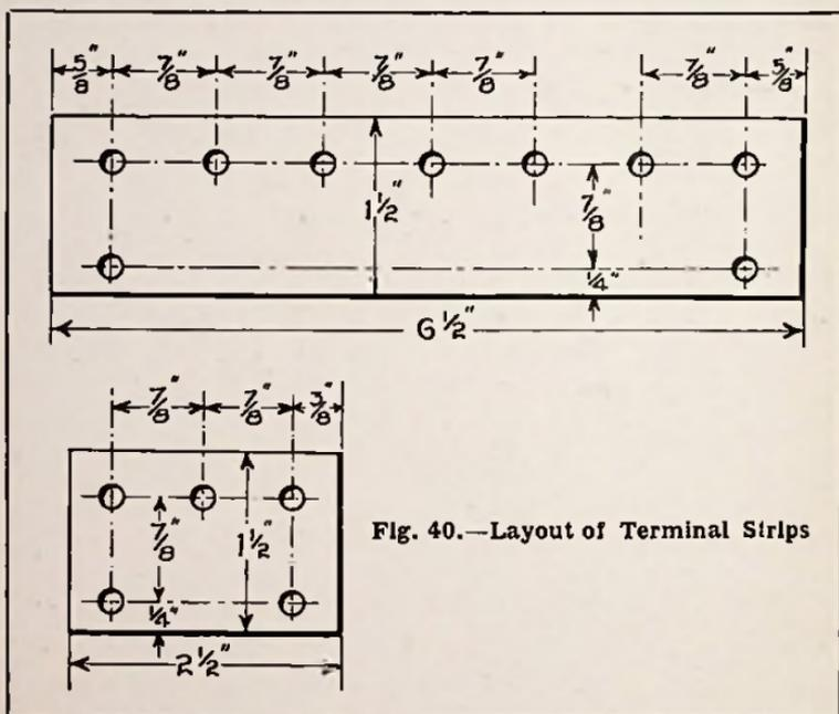
Fig. 40.—Layout of Terminal Strips
