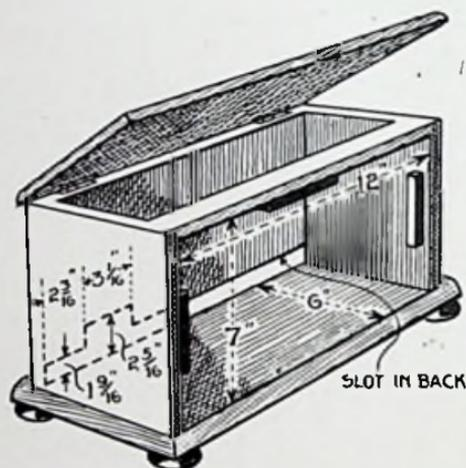
Fig. 42.—Cabinet for Oscillator and Detector Unit
