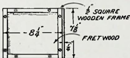
Fig. 21.—End Elevation of Cabinet
