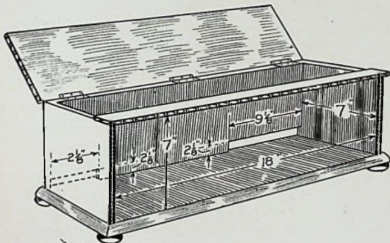
Fig. 47. Cabinet for I.F. Amplifying Unit
