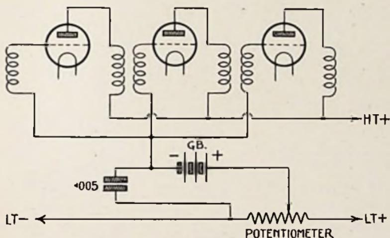
Fig. 6.—Introduction of Auxiliary Grid-bias Battery
