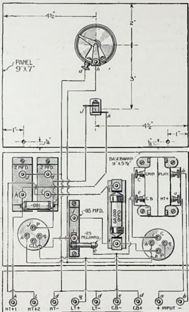
Fig. 50.—Combined Panel Layout and Wiring Diagram of L.F. Amplifier Unit
