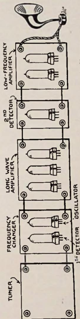
Fig. 3.—Super-heterodyne Receiver shown in Diagrammatic Form
