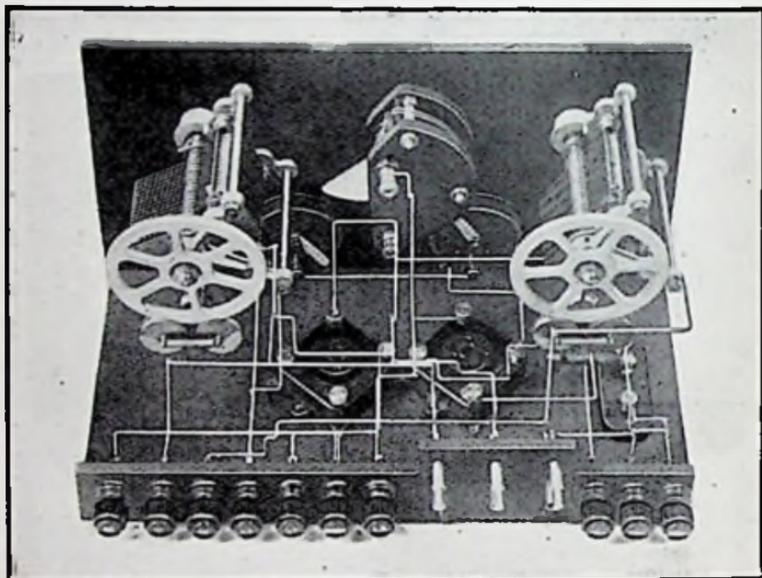
Fig. 38.—Photograph of Oscillator and Detector Unit, showing arrangement of Components on Baseboard
