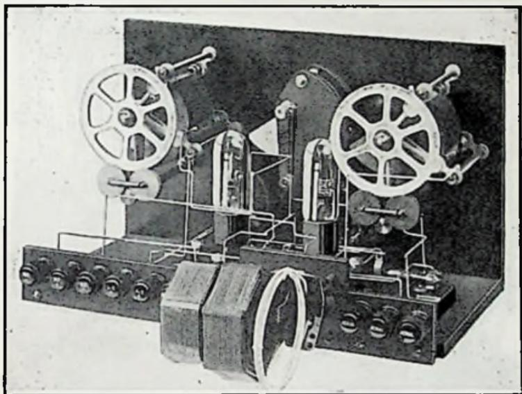
Fig. 38A.—Photograph showing Oscillator and "Pick-up" Coils in Position
