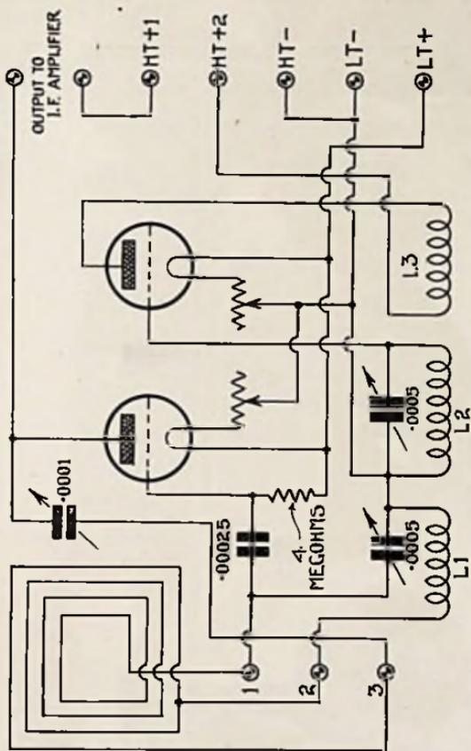
Fig. 35.—Circuit Diagram of the Oscillator and Detector Unit
