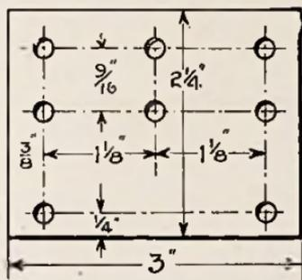
Fig. 41. Layout of Coil Strip
