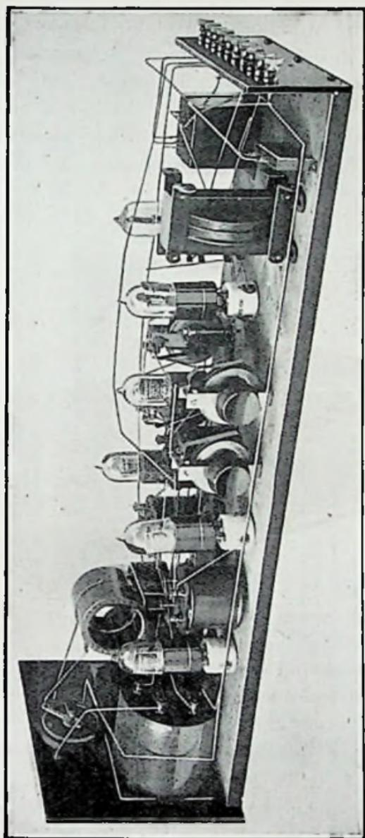
Fig. 27.—View showing Disposition of Components and Wiring
