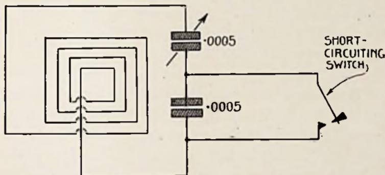
Fig. 7.—Sharp-tuning Arrangement
