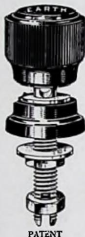
Type "B." The head and collar are insulated polished black "Bakelite." The names are neatly engraved in white letters on a black disc rigidly fixed to the stem, so that the name remains stationary in spite of the rotation of the clamping nut. The cross hole and slot in the stem facilitate connections above and below the panel.
