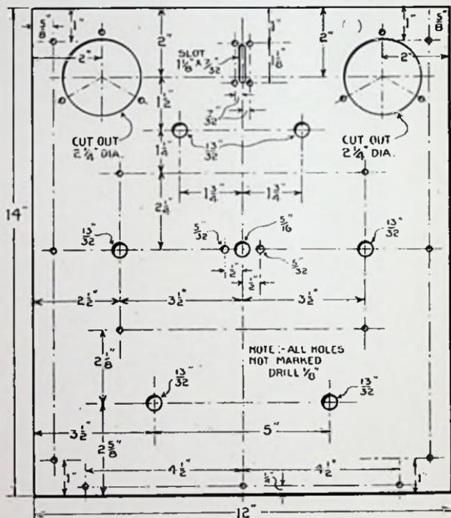
Fig. 57.—Layout of Front Panel
