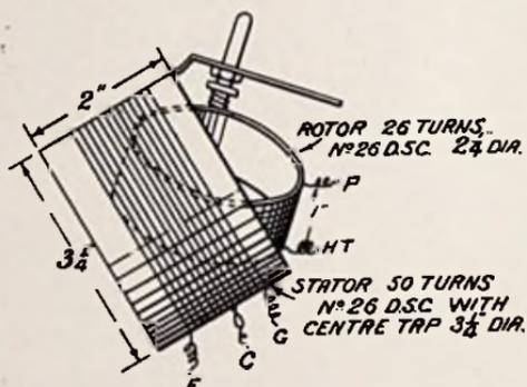
Fig. 16.—Oscillator Coupler
