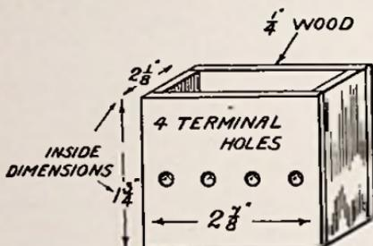
Fig. 14.—Box for Transformer
