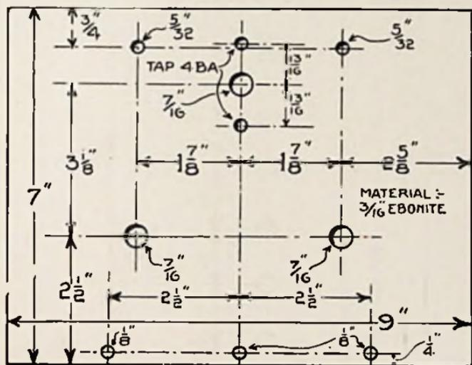
Fig. 29.—Layout of Front Panel of Seven-valve Super-het
