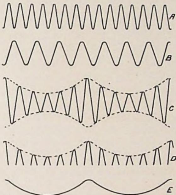
Fig. 1.—Diagrams Explaining the Principle of Super-heterodyne Reception: *A*, Current due to Carrier Wave; *B*, Current due to Local Oscillator; *C*, Combined Currents of Carrier and Oscillator; *D*, Resultant Currents Rectified; *E*, Resultant Lower-frequency Current
