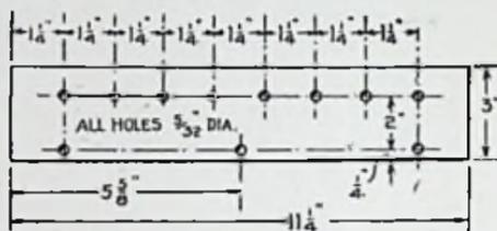
Fig. 54.—Details of Terminal Strip
